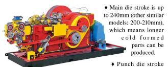
is up to 55mm (other similar models: 45mm), which means sophisticated parts with longer heads can be produced.
