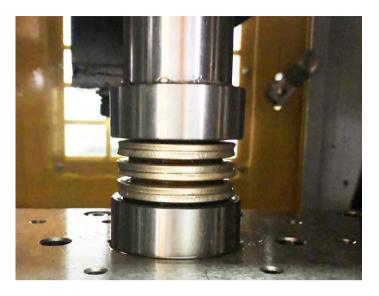
Zhou (Master of Engineering Degree in Germany) from Gui|in Ruite Testing Machinery Co., Ltd. to develop a new fatigue testing machine for spring washers. In terms of performance and software application, it is the first and leading equipment in China, which can carry out up to 400,000 times of fatigue testing for washers per day. By utilizing formulas, the equipment can automatically calculate the mechanical value after the corresponding specifications are entered in the software.
