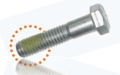
These bolts were replaced in the clutch and torqued into a tapped hole to the specifications given in the manual. The vehicle was placed in service, where a short time later, the bolts had head failures. No one thought to think that the epoxy would cause the failure.
