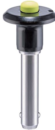
The clamp lock pins are available with mushroom-type knobs measuring 6 mm, 8 mm, 10 mm, 12 mm and 16 mm in diameter and with lengths ranging from 10 to 120 mm - depending on the version. The user can choose between two material options: a version made from stainless steel (1.4305) or a version constructed from precipitation hardened stainless steel (1.4542).
