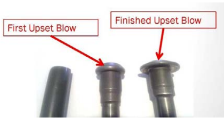
Figure 3: Example of a First and Finish Upset Blows
