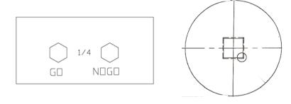
Square driver bits also need to be inspected for the same reasons a Hex bit requires inspection. A bad square driver bit can round out the screw recess resulting in an ineffective drive.
