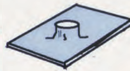
Standard extrusions are cut off with standard tapping screws leaving less than 1/2 pitch engagement
