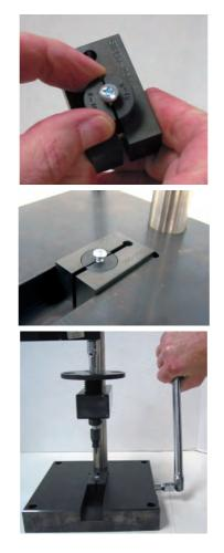
The appropriate style and size driver bit or socket is affixed to the lower end of the fixture's rotating shaft using an adaptor or bit holder if necessary. The upper arm is lowered until the bit or socket fully engages the screw's recess or head and the upper arm is firmly clamped to the fixture's main shaft. The driver or socket's height relative to the screw's head can be further adjusted by rotating the threaded adjustment wheel which houses the fixture's rotating shaft in the upper arm.
