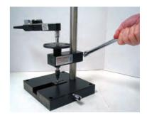
4. The torque wrench is firmly engaged in the upper end of the rotating shaft's female square recess. The wrenches indicator is set to "zero" before any torque is exerted on the wrench.
