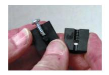
2. The collet is placed in the split collet holder. The split collet holder is then placed in the fixture's base so that the screw is positioned directly below the rotating spindle of the fixture. The clamp in the fixture's base is then tightened sufficiently to prevent the screw from turning in the collet when the torque is applied to the screw.
