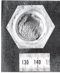
Fig.2.18 Fracture surface of anchor bolt of fatigue testing machine
