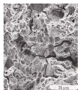
Fig.3.22 Results of observation by SEM of delayed fracture(6) (enlarged view of Fig.3.20)
