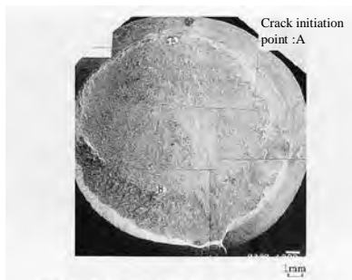
Fig.3.17 Delayed fracture of high tension bolt ( \sigma_B=1,100MPa )
