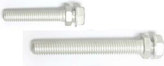
this safety screw, the torque value can be set in accordance with the clients' demand. Once the specified torque is reached, the first hexagon layer would automatically break to stop the operator's installation when the optimal performance of the fastener is reached, without worrying about over-tightening and rupture.
