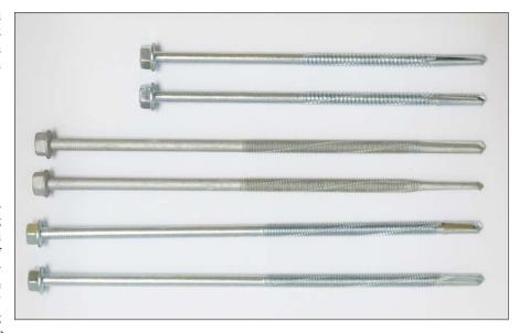
patented "crystal thread" will increase the size of the minor diameter to create spaces for wood particles to move while not affecting the pullout and lowers the drilling torque.
