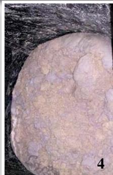
■ 1. Residue in the acid pickling trough
