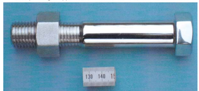
Fig. 10.11 Anti-loosening screw by shot peening effect
