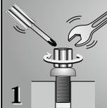
1 Tighten with spanner or cross-recess driver.
