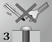
3 After the hexagon head moves off, removal is very difficult with the general tool, it's possible to prevent mischief and theft.
