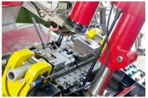
available on the market and eliminating the weaknesses. With a manufacturing process different from common self-drilling screw forming machines, YS250Z welds wire rods before pointing them. This creates more precise concentricity of screws and better torque performance than the conventional manufacturing process where pointing precedes welding. It is the innovative process exclusive to Yi Sheng Machinery.
