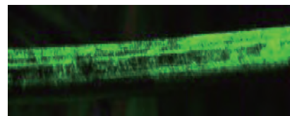
Fig. 3. Using magnetic powder to detect damages and found several bright lines
