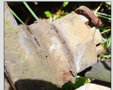
Fig. 5. Material damage by corrosion
