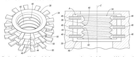
proximate the movable threaded element, thereby allowing the movable threaded element to move a predetermined distance within the cavity when torque is applied to the threaded fastener. The one or more spring-like members store elastic potential energy to prevent the loss of pretension of the threaded fastener that can be caused by heat or vibration. The invention also eliminates the need for a torque wrench when tightening the threaded fastener to a specified torque value.
