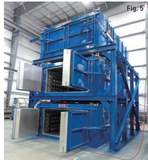
Fig. 4 Batch style oven with multiple doors (Courtesy of Wisconsin Oven Corp)
