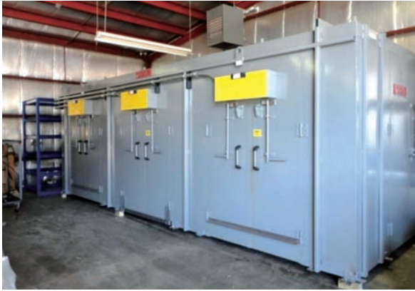
Fig. 6 Multi-door batch style oven for hydrogen stress relief (Courtesy of Wisconsin Oven Corp)
