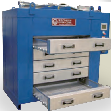
Figure 2 Five-drawer oven for hydrogen embrittlement relief of aerospace fasteners (Courtesy of Wisconsin Oven Corporation)
