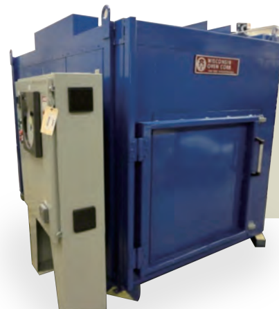
Figure 3 (a) Electric heated batch oven for embrittlement relief of fasteners (Courtesy of Wisconsin Oven Corporation)
