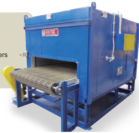
Figure 2 Five-drawer oven for hydrogen embrittlement relief of aerospace fasteners (Courtesy of Wisconsin Oven Corporation)
