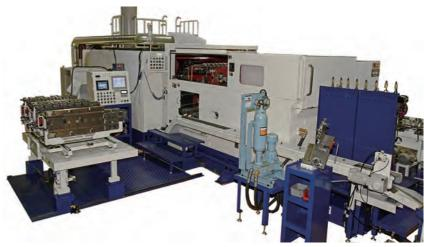
machine equipped with hydraulic servo mechanism which is able to realize closed forging, and back pressure forging. These machines are highly appraised and repeatedly purchased by customers.
