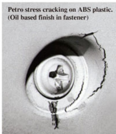
Fig. 5. Plastic Stress Cracking
