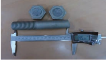
Pic. 4. ASTM A307B failure
