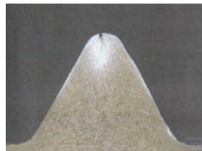
Pic. 2. Typical crack at the crest
