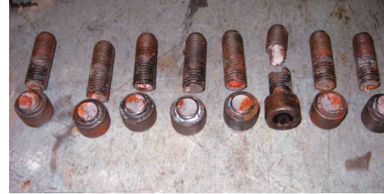
Pic. 5. Screws of fatigue fracture
