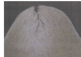
Pic. 3. 250µm crack
