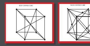
Also, as temperatures increase, the iron's lattice structure changes from a face centered cubic (f.c.c.) to a body centered cubic (b.c.c.). Cold worked materials should be heat treated more slowly than stress-free materials to avoid distortion.
