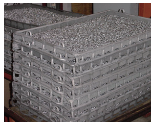
Figure 9 Typical Load of 17Cr4Ni Fasteners for Vacuum Heat Treatment (Photograph Courtesy of Solar Manufacturing)
