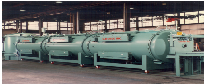
Figure 7 Typical Continuous Vacuum Heat Treat Equipment Servicing the Automotive Industry (Photograph Courtesy of C. I. Hayes)
