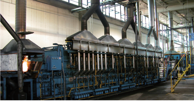
Figure 4 Typical Atmosphere Heat Treating System for Fasteners (Photograph Courtesy of Williams Industrial Service, Inc.)
