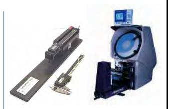
an inch depending on the size and type. One way these measurements can be done is optically on an optical comparator or tool makers microscope, but this can be time consuming when there are large quantities and different sizes to check. Caliper length measurements are probably the most commonly used method, because it is relatively quick, however it is often difficult to get good repeatability. There are also several specialty type length gages that will help increase speed and repeatability.
