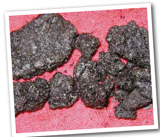
Figure 2 Sludge Buildup in a Quench Chute
