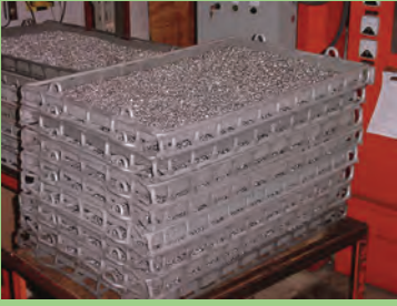
Figure 4 Load of Custom 630 Fasteners for Solution Heat Treatment and Aging (Photograph Courtesy of Solar Atmospheres Inc.)
