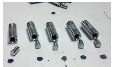
Picture A: Loosened dilating plugs and plastic plugs.
