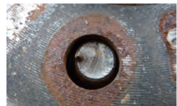
Fig. 3. Multiple fatigue initiation sites
