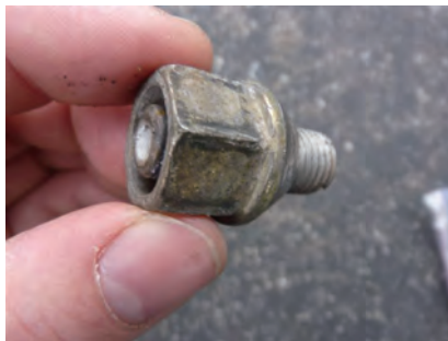
Fig. 6. Impact wrench effect on a nut
