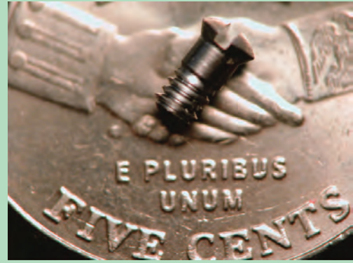
Figure 5. Hip Repair Screw After Heat Treatment (Photograph Courtesy of Midwest Thermal-Vac)
