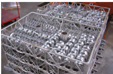
Figure 2. Load of Knee Implants after Heat Treatment (Photograph Courtesy of Solar Atmospheres, Inc.)
