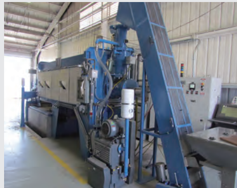
Figure 2. Shaker Hearth Furnace for the Heat Treatment of Titanium Fasteners (front end) (courtesy of DF Industries)
