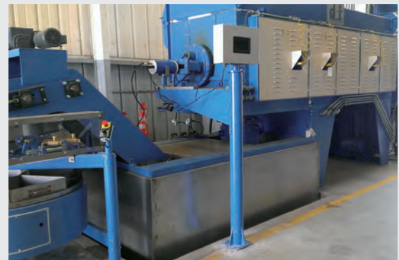
Figure 3. Shaker Hearth Furnace for the Heat Treatment of Titanium Fasteners (rear end) (courtesy of DF Industries)
