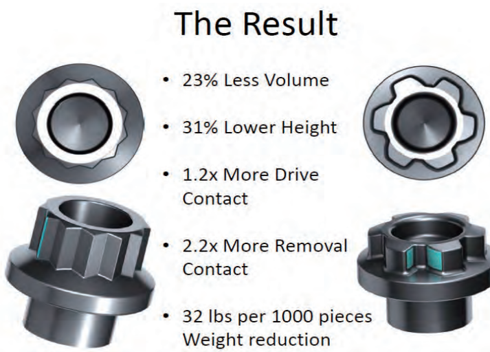
Fig. 2 Comparison Between Phillips Screw Company's Conventional Fastener and Its Optimized Fastener Data source: "Optimizing Fasteners for Weight Reduction, Serviceability and High-Speed Assembly", Michael Mowins, Phillips Screw Company; arranged by MII of MIRDC (Aug. 2015)
