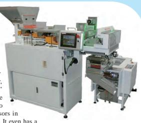
foothold in the food industry, because surprisingly its Digital Area Counters are used to count food materials, frozen foods and even plant seeds besides fasteners. This proves Digital Area Counters can count many types of products with complex shapes. At this point, you must be curious what is so accurate and versatile about Digital Area Counters.
