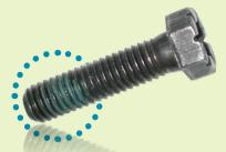
These bolts were replaced in the clutch and torqued into a tapped hole to the specifications given in the manual. The vehicle was placed in service, where a short time later, the bolts had head failures. No one thought to think that the epoxy would cause the failure.
