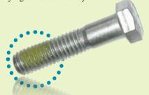
These epoxy type of locking aides are very good if used properly. Most users will not employ a torque wrench to tighten their fasteners, so these epoxy coated fasteners will work well. However, caution must be observed when using any air impact assembly tools, as these fasteners will not have sufficient friction to cause these tools to stall and the fasteners will be either stretched into yield or have their threads stripped.
