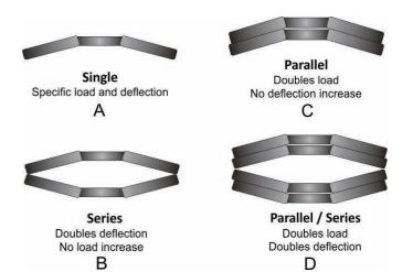
One of the unique properties of these spring washers is their ability to produce different loads and / or deflection by how they are arranged; single, series, parallel or stacked.
