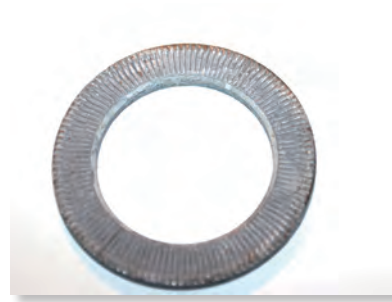
Fig. 6. Ridges on the washer
