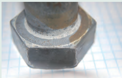
Fig. 5. Illustrating embedment of the ridges into the bolt head
