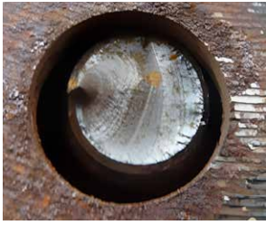
Photo 3. Metal fatigue fracture of a wheel stud
