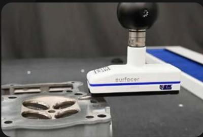
LK Metrology has introduced the SURFACER SRP, a high-resolution surface roughness probe designed for use on any coordinate measuring machine (CMM) with a standard probe head. With a resolution of one micron, this plug-and-play probe allows manufacturers to integrate surface roughness measurement directly into the CNC measuring cycle without needing secondary inspection. This streamlines inspection by combining multiple measurement processes into a single setup, saving significant time and cost.
