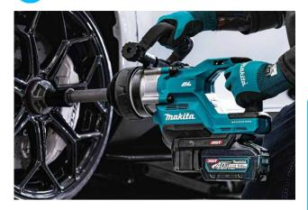
The 40V max XGT 4-Speed High-Torque 1" Impact Wrench (model GWT10) is engineered by Makita specifically for demanding tasks such as removing wheels and attachments on heavy machinery and trucks. This cordless square-drive wrench eliminates the need for bulky air compressors and is said to outperform pneumatic models, offering up to 2,950 ft-lbs of fastening torque and 2,320 ft-lbs of nut-busting torque.
